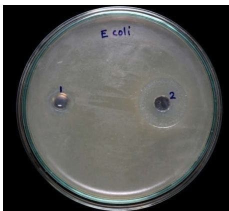
Fig-7. Image of agar diffusion of chitosan composite against E-coli (standard sample MTCC 1687)
