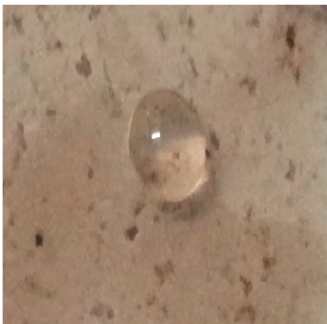
Fig-3. Lotus leaf effect-Image of water drop on the film surface
