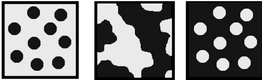
Figure 1.4 Relative amount of polymer B in the immiscible polymer-polymer system of A and B.
